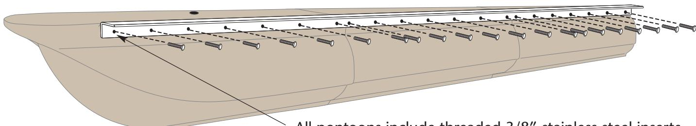
All pontoons include threaded 3/8" stainless steel inserts to accommodate bolts.
